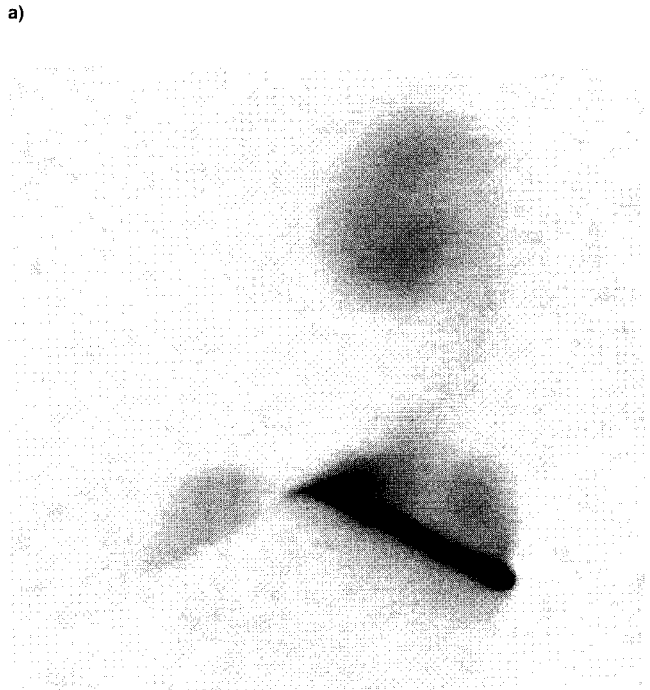
Fig. 15 Light sheet negative flow visualization, \alpha = 40 deg: a) no blowing and b) maximum blowing.
